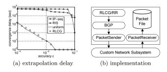
Figure 3: Extrapolation delay and IRLscanner implementation.
